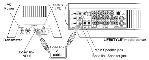
Note: If another product is already connected to the Bose link Speaker jack on the media center, disconnect it there. You can use the wireless audio link to replace this wired connection. Or, to continue using this connection, reconnect the cable to the jack labeled Bose® link OUTPUT on the transmitter connection panel (Figure 4).
